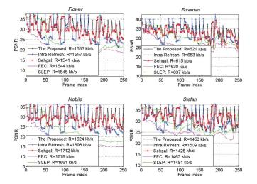
Fig. 22. PSNR comparison of different error resilient schemes.
