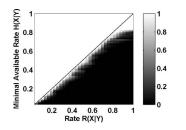
Fig. 6. Correlation of a combination of H(X|Y) and  $P_e$  versus the WZ bitrate R(X|Y).
