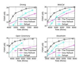
Fig. 18. RD performance of *anchor frames* with packet loss ratio 8% (high resolution).
