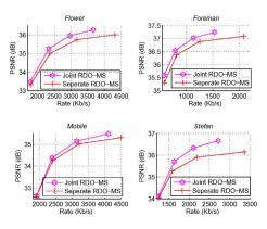
Fig. 14. Performance gain of joint source-channel RDO-MS.
