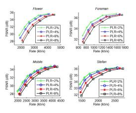
Fig. 20. RD performance of *anchor frames* with different packet loss ratio (PLR).
